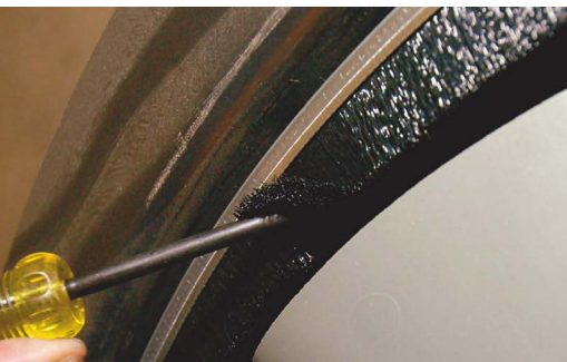
The brush ring between the shroud and fan blades closes up this annular space for more efficient airflow and protects the fan blades when the engine flexes. (This is not an actual installation.)
