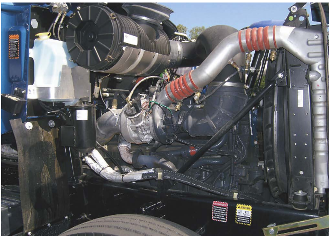
The twelve-liter ASET engine pulled more strongly than its torque and horsepower numbers suggest, while its variable-geometry turbo whistled happily.
