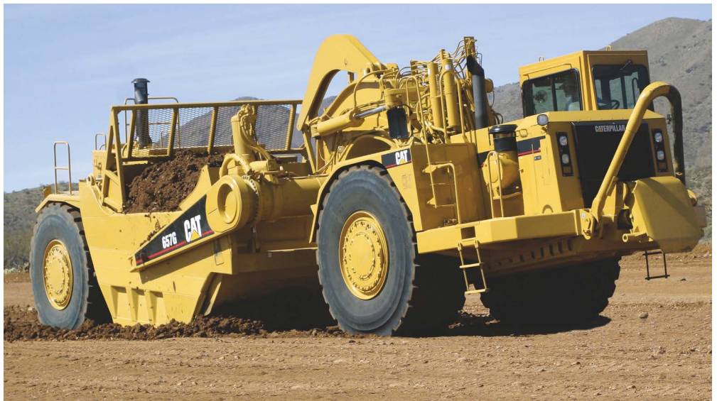
Caterpillar’s latest and largest G Series scraper — the 657G — features Tier III-compliant ACERT engines. Dual horsepower capabilities of 451/410 at the rear and 600/564 at the tractor produce more power in higher gear ranges for fast cycle times.
