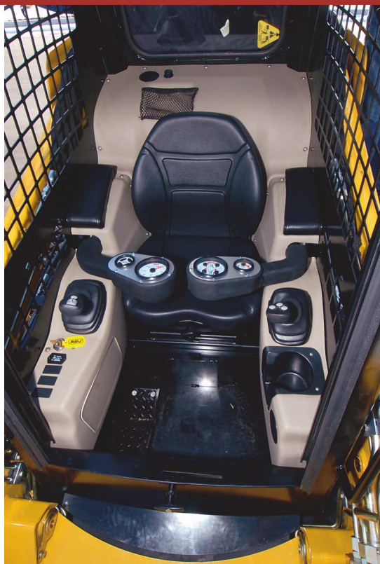
New features in the SR-Series operator's station include a two-piece lap bar with integral gauges, redesigned joystick controllers, new suspension seat, set-position foot throttle, variable low-flow control and selectable bucket positioning.
